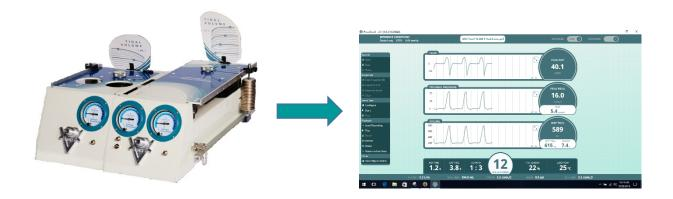
This system is intended to provide an adjustable, passive, mechanical simulation of human lungs and allow for the interpretation of data from the simulated lungs and airway during ventilation.
