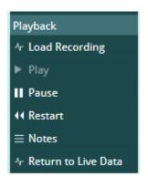
Pause – Stops the playback at its current point and freezes the waveform and numerical display. The Play selection then becomes active.
