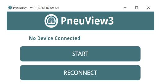
If the Lung Simulator is turned On and the USB data cable is properly connected, "RECONNECT" may be selected to launch the full Setup Screen.
