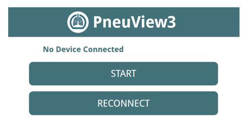
If the lung is turned on and the USB data cable is properly connected, "RECONNECT" may be selected to launch the full PneuView Setup Screen.
