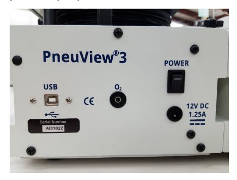
Step 3: Flip the switch on the PneuView Module to the On position. A green LED indicator on the switch will light up to confirm power to the unit.
