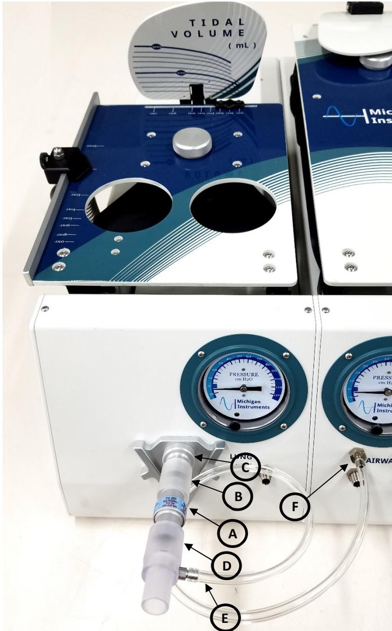
1. Select one PneuFlo resistor (A) to simulate total airway resistance and connect it to the 15mm airway adaptor (B).
