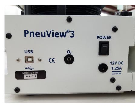
Step 3: Flip the switch on the PneuView Module to the On position. A green LED indicator on the switch will light up to confirm power to the unit.
