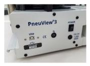
The PneuView Electronic Module is the interface between the PneuView lung and the PneuView software. This module is built into the lung as shown on the left. It incorporates pressure transducers, environmental sensors, signal conditioning and analog-to-digital converter circuitry. The Electronic Module communicates with PneuView software installed on a computer.
